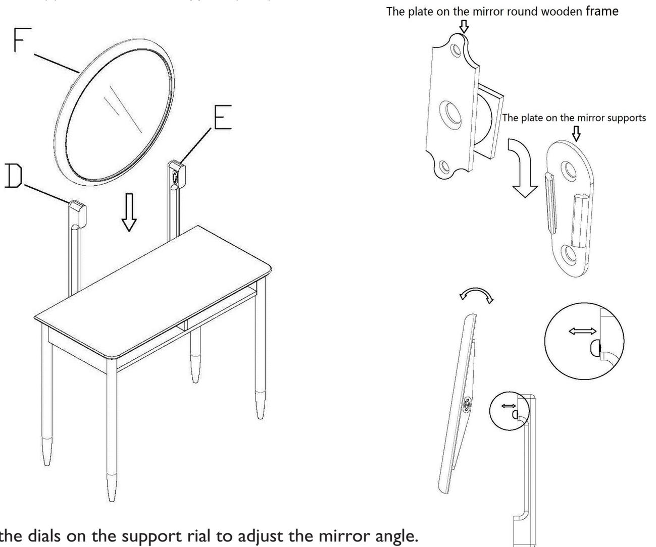
Rotate the dials on the support rial to adjust the mirror angle.
