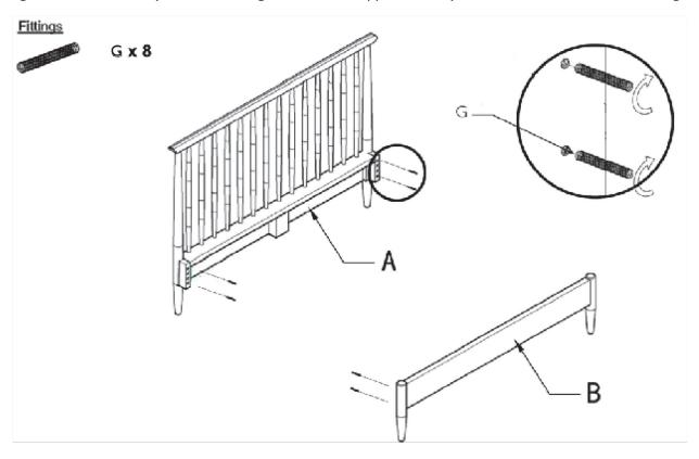
2. Making sure the holes in the side rails, C, are facing upwards, AND you have the Left and Right rails, (see page 2) on the corret sides, locate these side rails onto the protruding threads on the headboard and foot board. As you do this, slide a half moon washer onto the thread when it comes through into the circular hole in the side of the rail, then screw on one of the 8 nuts FINGER TIGHT ONLY. Repeat with the other 3 corners.
