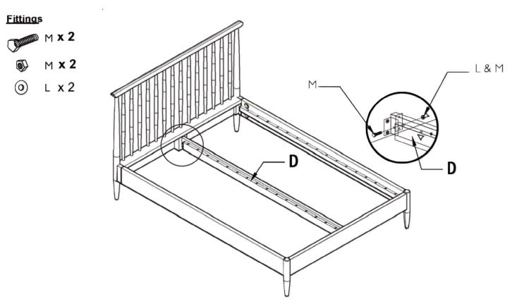
5. Push a plastic cap onto each end of a slat and with the peg facing downwards push the slat into the pre drilled holes as shown below. Repeat for all the slats.
