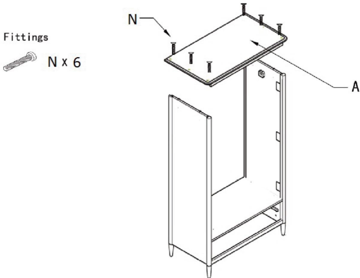
4. To increase the overall strength, Using 4 of the 30mm screws (I) attach the side panel rails front and back to the top of the wardrobe through the pre drilled holes provided, see below. Attach the door panels onto the side panels as shown below.
