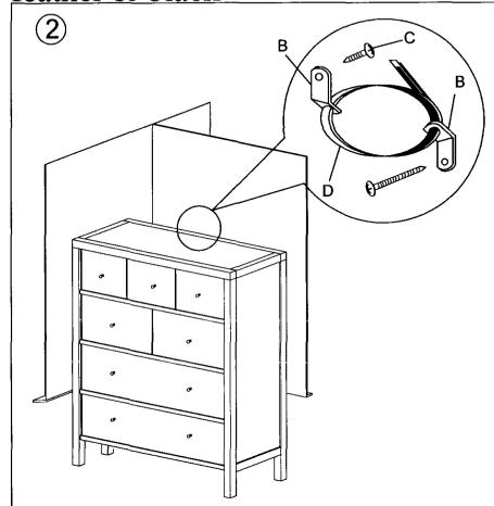
IMPORTANT: The screw supplied with the anti topple strap is to be used only for fixing the anti topple strap to the furniture. In addition to this you will need to choose a screw or fitting which is suitable for securing the strap to the kind of wall that you have. If you are unsure about what type of screw to use please contact your local hardware store.
