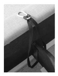
Step 2: Thread loop 2, between the metal frame with slats (Part 1) and the frame linking bracket (Part 2). Wrap loop 2 around metal frame with slats, and pass the end back though the loop and pull tight.
